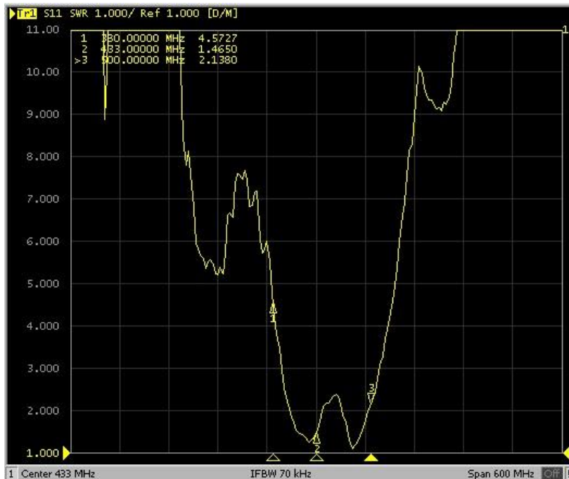
Figure 2 - VSWR tested with 30cm cable length
