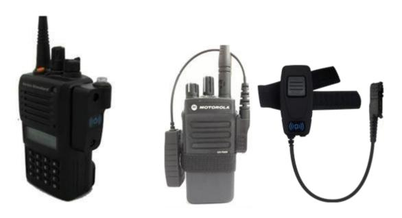
Each BT dongle is fitted with 2 Bluetooth channels, 1 for pairing an audio device, the 2<sup>nd</sup> pairing an optional Bluetooth wireless PTT shown below (JB-PTT). There is also a PTT button on the BT dongle.
